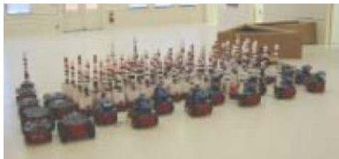
Figure 5 - The multi-robot team used in [18]. Two types of robots can be seen: leader robots and sensor robots.
